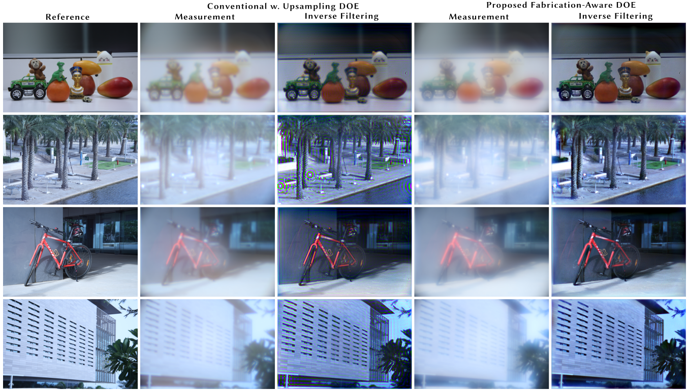
Fig. 14. Experimental Validation of Fabrication-aware Broadband DOE for Imaging. We capture diverse indoor and outdoor scenes with both conventional nearest up-sampling DOE and proposed fabrication-aware DOE (column 1, 2, and 4). To visualize the discrepancy between the designed PSF and fabricated PSF, we conduct a Wiener filtering using simulated PSF on the experimental captured scenes assuming high SNR ( \gamma = 5 \times 10^{-4} ). Our proposed fabrication-aware design yields high-fidelity results, while the conventional nearest up-sampling results in images with severe chromatic aberration, ringing artifacts, and elevated noise.
