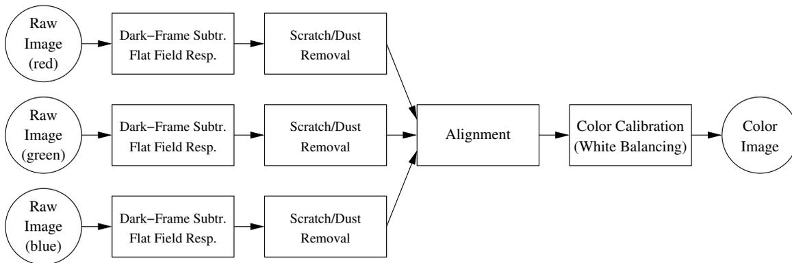
**Figure 6.** Processing pipeline for color images: first the individual color planes are treated with the calibration stages known from the B&W process. Then, the color planes are aligned, and a color calibration using ICC profiles is performed. Note that the gamma correction is now implicitly performed in the color calibration stage.
