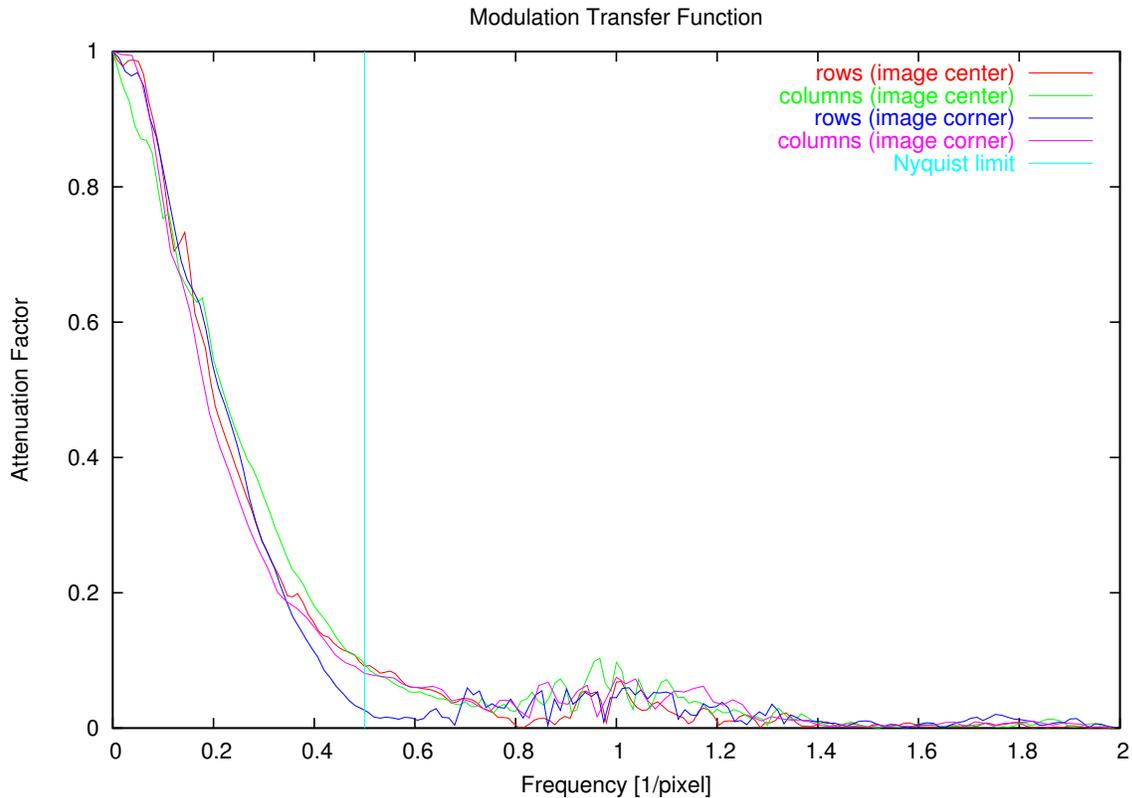
**Figure 7.** The modulation transfer function for the rows and the columns of our optical system
