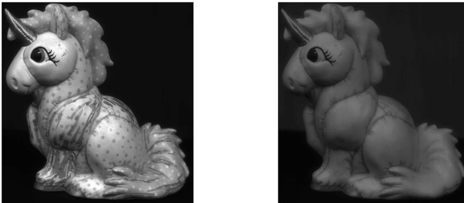
**Figure 5.** Comparison of a black&white photograph (left) with an infrared photograph (right). Note that except for the black color of the eye, the effect of different paints is almost completely removed in the infrared image.
