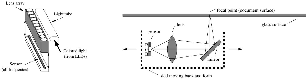
**Figure 2.** Left: Design of a scanner with the LIDE (LED in Direct Exposure) technology. Right: Design of a conventional flatbed scanner.
