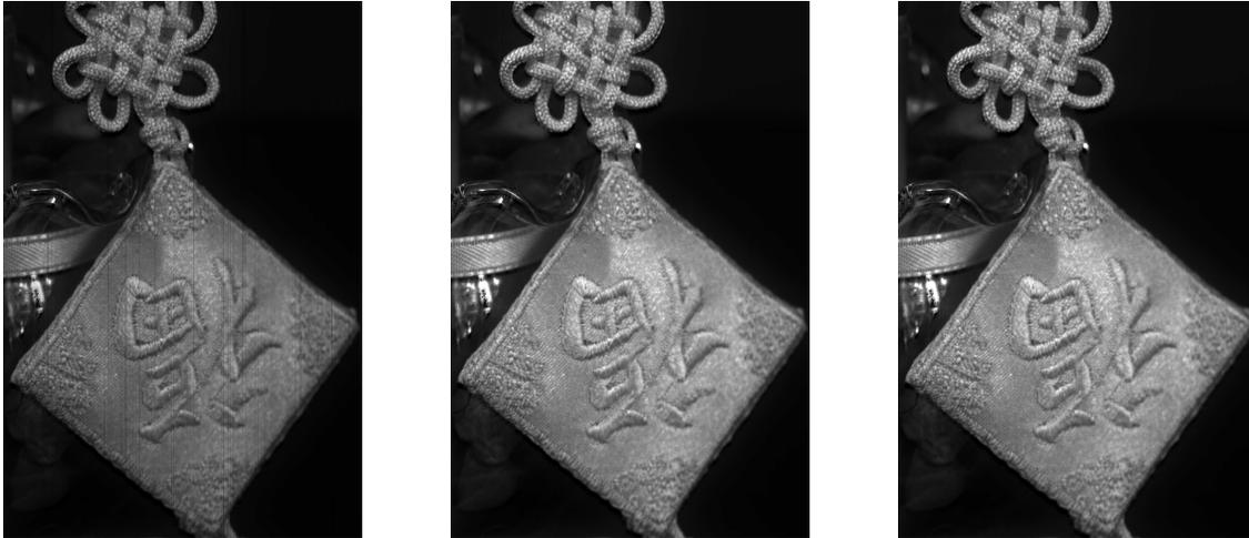
**Figure 4.** Effect of the black&white calibration step. Left: raw sensor data. Center: after dark current subtraction and flat-fielding. Right: calibrated image after interpolating faulty columns.
