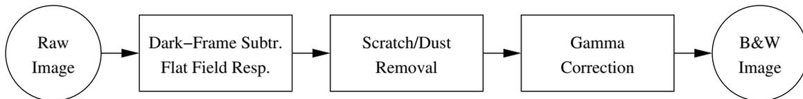
**Figure 3.** Processing pipeline for B&W images: first, dark-current noise and flat-field response are calibrated with a single linear mapping. Then, broken columns in the image are interpolated. Finally, gamma correction yields the end result.
