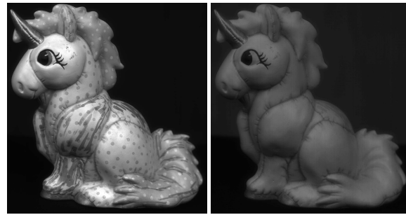
Figure 6: Comparison of a black&white photograph (left) with a near infrared photograph (right). Note that except for the black color of the eye, the effect of different paints is mostly removed in the NIR image.
