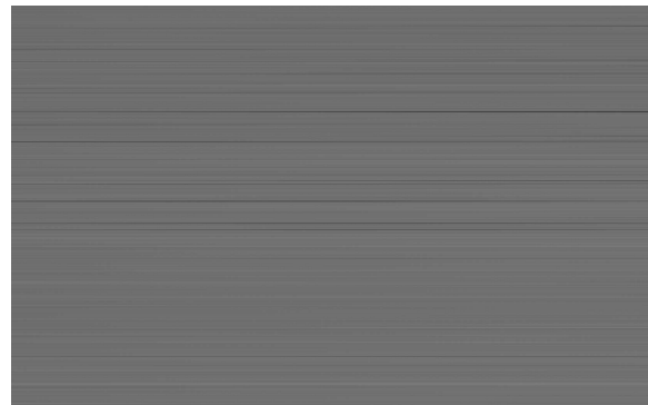
Figure 4: Enhanced raw scan of a white surface illustrating both position-dependent and position-independent sensor artifacts.
