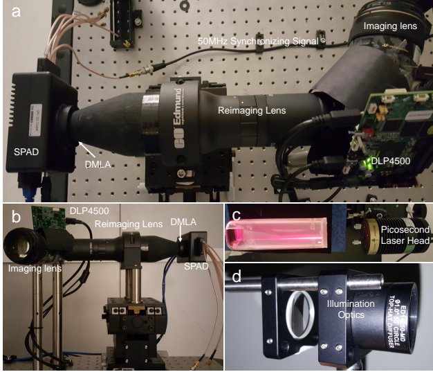
Figure 7. Prototype of Imaging System: (a) Top view of our imaging system. (b) Side view of our imaging system. (c) Scene of light propagating in the milked water. (d) Illuminating optics with a diffuser and a 30mm biconvex lens.
