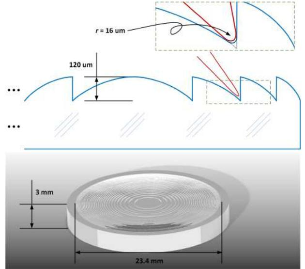
Fig. 4. Illustration of the rounded head region of the turning tip (top) and the 3D layout of our prototype lens (bottom).
