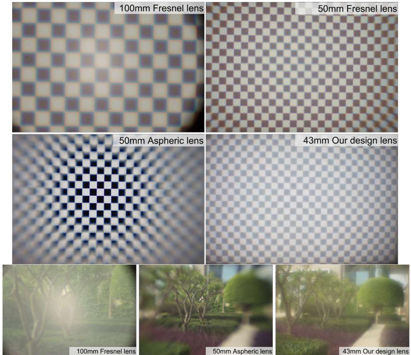
**Fig. 9.** Comparison results of a chessboard target (top) and a wild scene (bottom) captured by Fresnel lenses (aperture 8mm), an aspherical lens(aperture 23.5mm), and our prototype lens(aperture 23.5mm).
