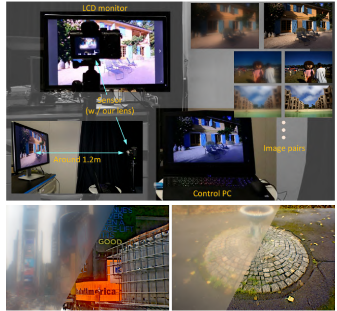
Fig. 6. Top: Illustration of our display-capture setup for preparing the training data set. Selected displayed and captured image pairs are shown as inserts; Bottom: Results on testing set images captured by our lenses. For each example we show the degraded measurement and reconstruction side-by-side.
