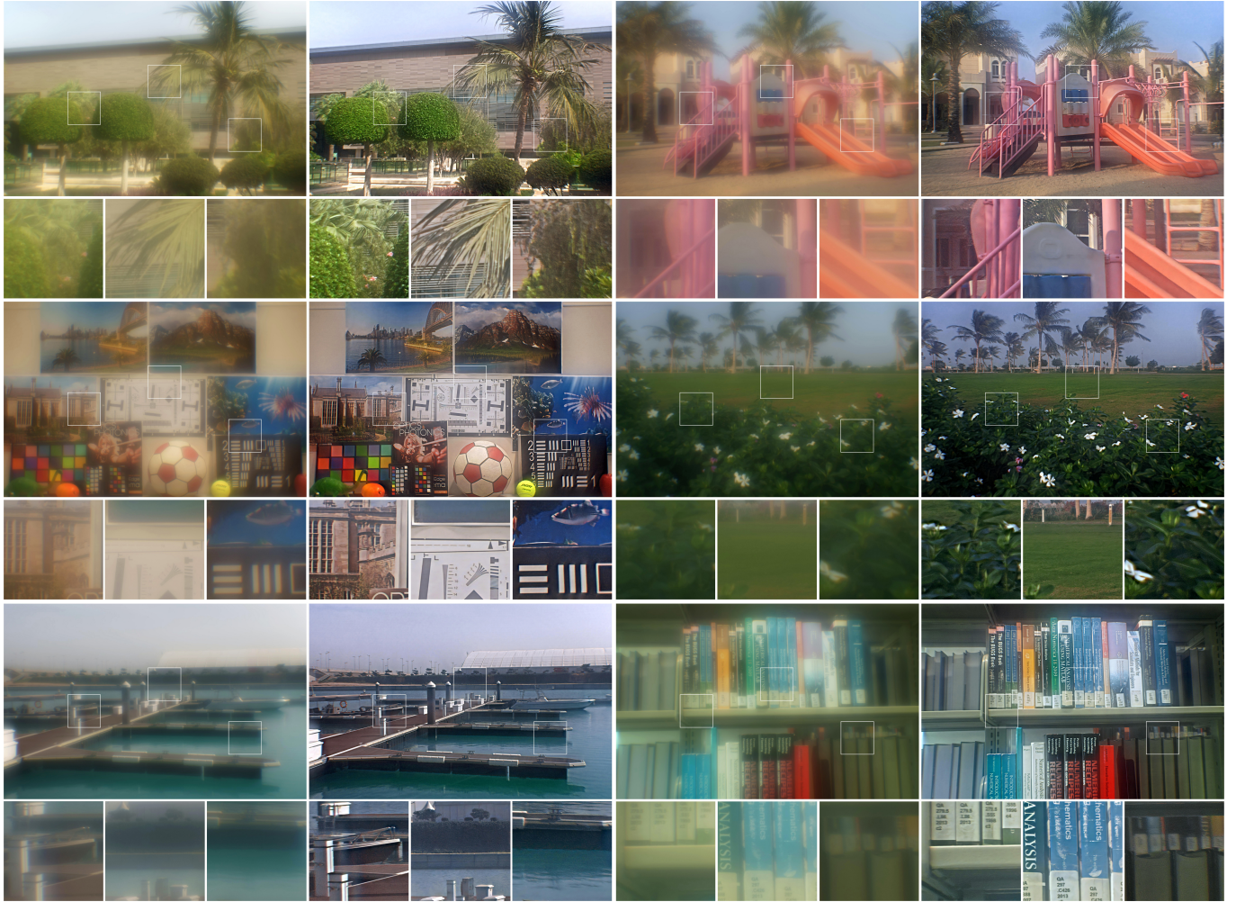
Fig. 11. Experimental results of dual-surface lens design (first two rows) and that of single surface lens design (third row) on real word scenes. For each pair, we show the degraded measurement and the reconstruction result. The exposure time for these images are set 0.8, 125, 0.5, 1.25, 0.5, 0.4 ms with ISO 50. Refer to supplementary document for more real world results.
