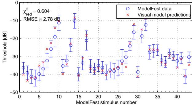
**Figure 7:** Visual model predictions for the **ModelFest** data set. Error bars denote standard deviation of the measurements. The  $R$  value is the prediction mean square error and  $\chi^2_{red}$  is the reduced chi-square statistic.
