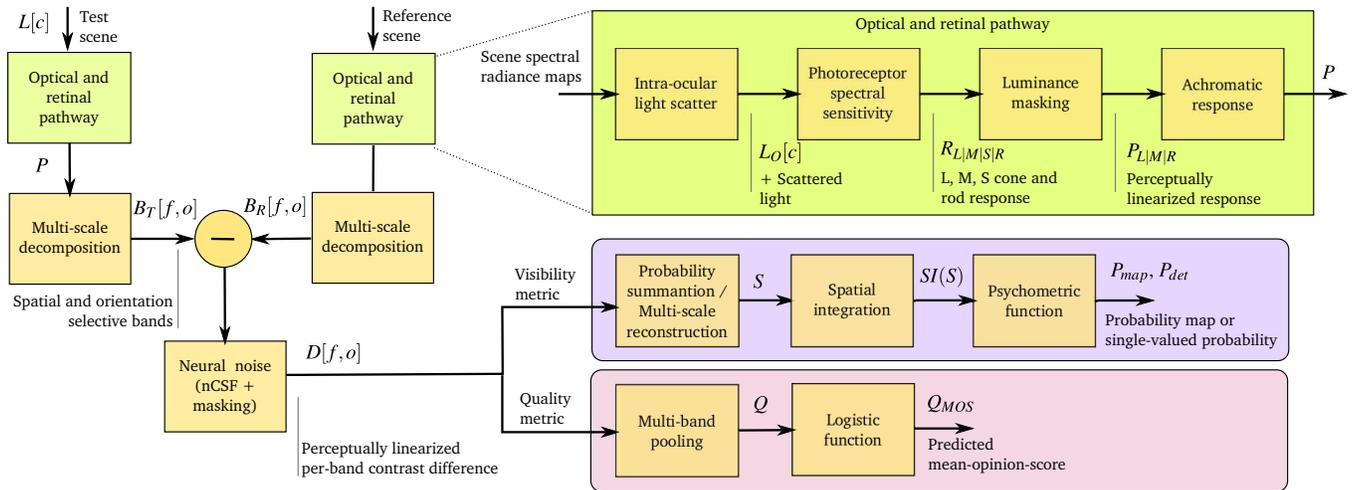
**Figure 2:** The block-diagram of the two visual metrics for visibility (discrimination) and quality (mean-opinion-score) predictions and the underlying visual model. The diagram also summarizes the symbols used throughout the paper.
