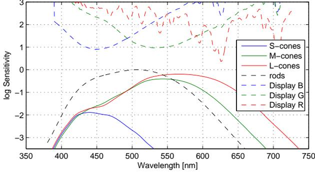
**Figure 4:** Spectral sensitivities of the photoreceptors from [Stockman and Sharpe 2000] and [CIE 1951] (bottom). The curves in the upper part of the plot show the measured emission spectra for a CRT display (inverted and arbitrarily scaled to distinguish from the bottom plots).
