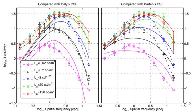
**Figure 6:** The CSF measurement results compared to two popular CSF models by Daly [1993] and Barten [1999]. The Dashed lines represent our measurements and the solid lines the two compared models. The model parameters, including stimuli size, were set to match our measurements. The predictions of both models differ from the measurements probably because of different experiment conditions.
