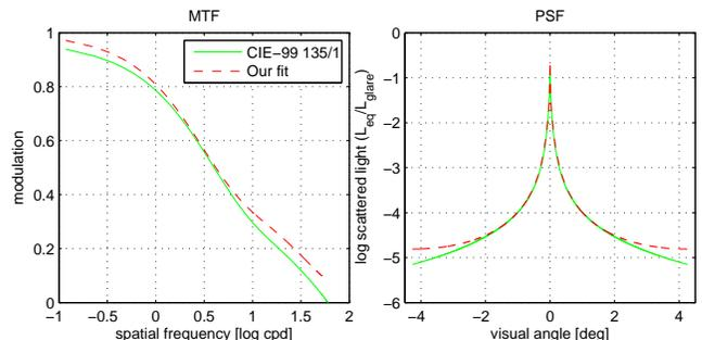
**Figure 3:** Comparison of our fitted intra-ocular light scatter model with the model from the CIE-99 135/1 report [Vos and van den Berg 1999]. Left panel shows the modulation transfer function of the eye and the right panel its corresponding point spread function. The MTF for the CIE-99 135/1 glare spread function has been computed by creating a densely sampled digital filter and applying the inverse Fourier transform.
