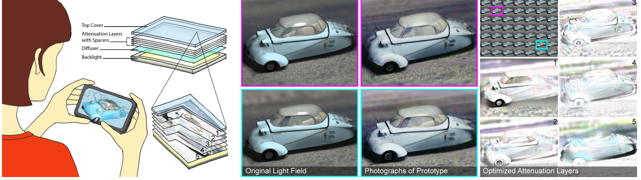
Figure 4. Layered 3D: Inexpensive, glasses-free light field display using volumetric attenuators. (Left) A stack of spatial light modulators (e.g., printed masks) recreates a target light field (here for a car) when illuminated by a backlight. (Right) The target light field is shown in the upper left, together with the optimal five-layer decomposition, obtained with iterative tomographic reconstruction. (Middle) Oblique projections for a viewer standing to the top left (magenta) and bottom right (cyan). Corresponding views of the target light field and five-layer prototype are shown on the left and right, respectively. Such attenuation-based 3D displays allow accurate, high-resolution depiction of motion parallax, occlusion, translucency, and specularities, being exhibited by the trunk, the fender, the window, and the roof of the car, respectively.
