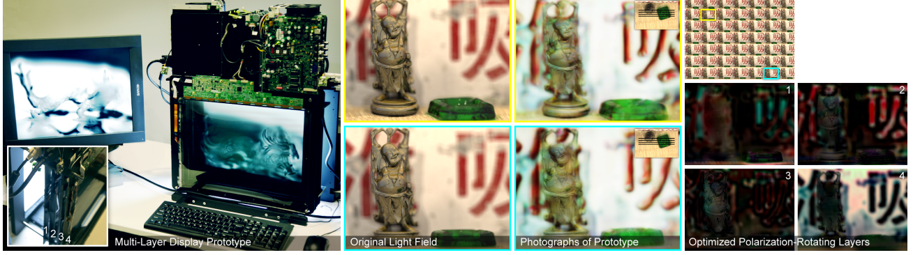
Figure 5. Polarization Fields: Dynamic light field display using multi-layer LCDs. (Left) We construct an optically-efficient polarization field display by covering a stack of liquid crystal panels with crossed linear polarizers. Each layer functions as a polarization field rotator, rather than as a conventional optical attenuator. (Right, Top) A target light field. (Right, Bottom) Light fields are displayed, at interactive refresh rates, by tomographically solving for the optimal rotations to be applied at each layer. (Middle) A pair of simulated views is compared to corresponding photographs of the prototype on the left and right, respectively. Inset regions denote the relative position with respect to the display layers, shown as black lines, demonstrating objects can extend beyond the display surface.
