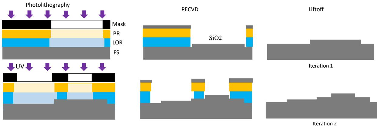
Figure 1. *Fabrication of 16 level fresnel lens.* Each iteration creates 2-level microstructures on the previous profile by applying lift-off lithography followed by SiO<sub>2</sub> deposition. By repeating the fabrication cycle 4 times, one can obtain 16 levels fresnel lens. PR: photoresist. LOR: lift-off resists. SiO<sub>2</sub>: Silicon dioxide. FS: fused silica. UV: ultra violet.
