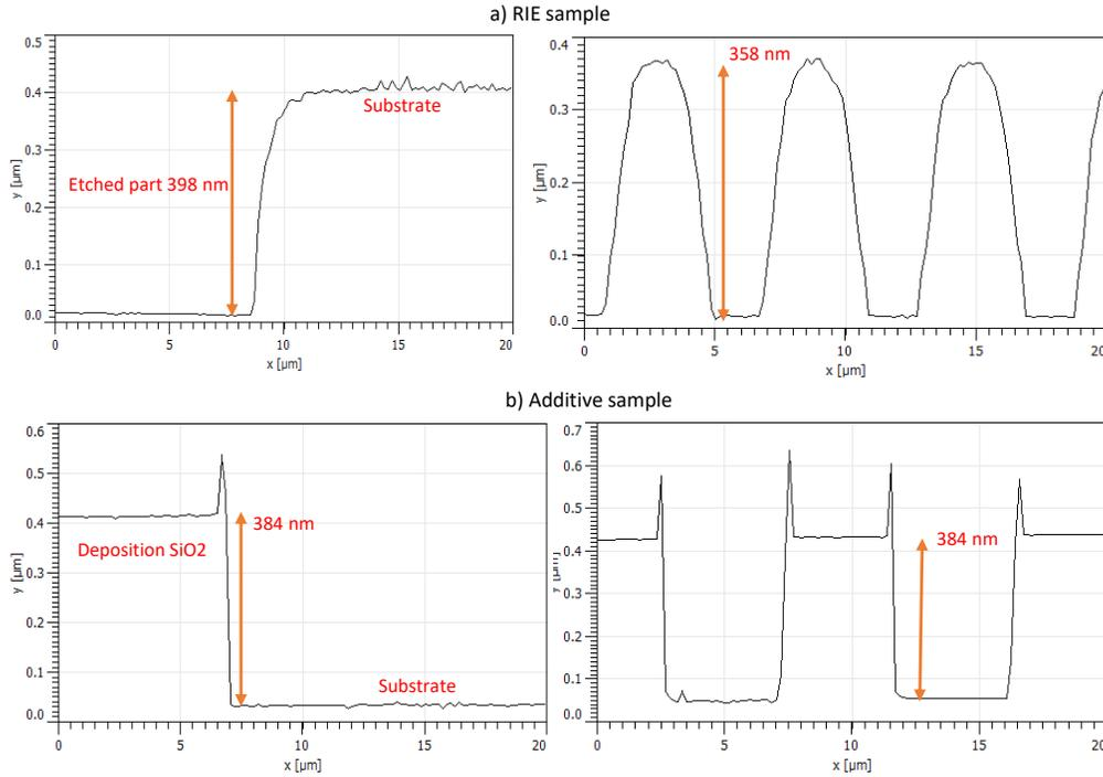
Figure 4. AFM characterization using Bruker Dimension Icon Atomic Force Microscope System. The X-axis represents the DOE feature size, and the y-axis represents the DOE depth.
