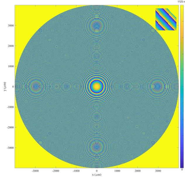
Figure 2. The designed Fresnel lens; Discretized 16-level height profile.
