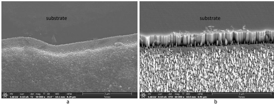
Figure 3. SEM characterization using Nova NanoSEM630 machine: a- additive sample, b-RIE sample.
