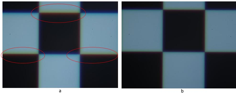
Figure 5. Optical characterization: a-Image capture with the additive lens, b-image captured with RIE lens .
