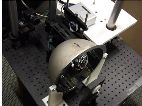
Figure 4. Photograph of the proposed BRDF acquisition setup including a camera, a projector, a beam-splitter, and two curved reflectors mounted on a 40 cm × 40 cm optical bench.
