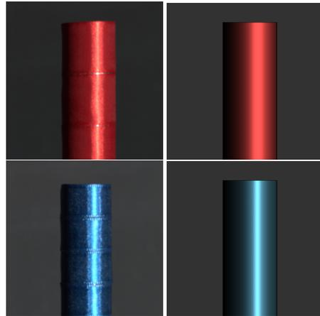
Figure 9. Visual comparison of two kinds of acquired satin samples wrapped around a cylinder as lit by a point source against real photographs. Left column: Photographs of the red and blue satin samples. Right column: Rendering of the D-BRDF fits.
