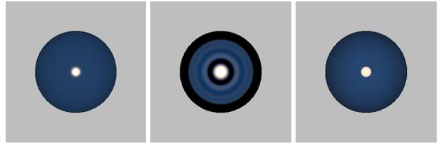
Figure 3. An illustration of the suppression of ringing through fitting analytical BRDF models. Left: original acrylic blue paint BRDF acquired by Matusik et al. [22]. Center: 10<sup>th</sup> order zonal reconstruction, rendered after transformation into SH, exhibiting severe ringing artifacts. Right: Corresponding D-BRDF fit to the zonal reconstruction.
