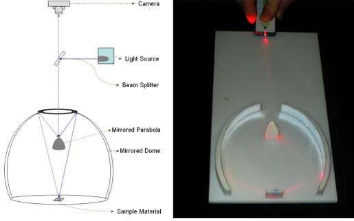
Figure 1. Left: Physical setup of our reflectance acquisition device. A camera focused on the mirrored components views a zone of reflected directions. A projector illuminates the corresponding zone of incident directions using a beam splitter. Right: A prototype demonstrating the concept in 2-D. Here, we focus illumination on the mirrored components using a laser pointer and observe that the beam bounces back to its origin.
