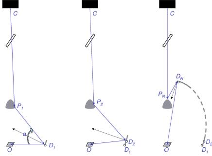
Figure 5. Iterative process for designing the profile of the reflective dome for a fixed convex parabolic reflector.
