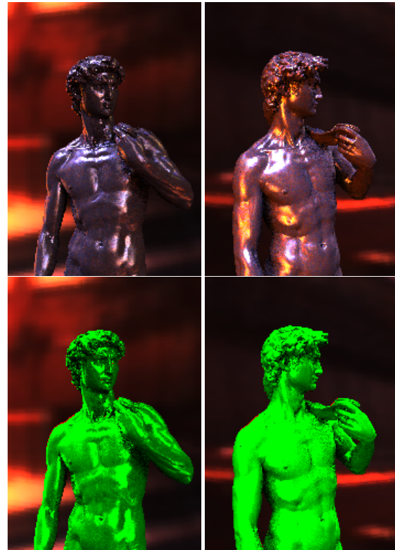
Figure 6: SMC sampling for a camera animation sequence with the David model in the Grace Cathedral EM. Top row: Images rendered with SMC sampling for dynamic viewpoints. Bottom row: False color visualization of bidirectional samples (red) and SMC samples (green).
