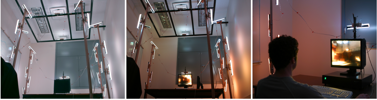
Figure 11: Left: photograph of the room housing our system, with all lights switched on. Center: illumination programmed to resemble the Grace Cathedral environment. Right: A user viewing the Grace Cathedral environment on an HDR display in a room illuminated by our system. Note how the room illumination is consistent with the virtual environment shown on the screen.
