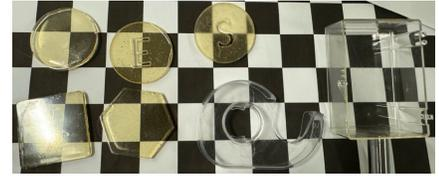
Fig. 13. **Proposed 3D Photoelasticity experimental dataset.** We acquire multi-axis polariscope measurements for a variety of 3D shapes and force application conditions. (a) depicts examples from the dataset with the measurement  $\cos \delta_{eq}$ . The photoelastic test specimen are created from epoxy resin and shown in (b).
