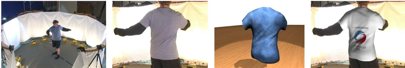
**Figure 1:** Left to right: an actor performing in the capture setup; one of sixteen views from the camera array; reconstructed T-shirt geometry; the real T-shirt is replaced by a rendering of the captured geometry with different appearance characteristics.
