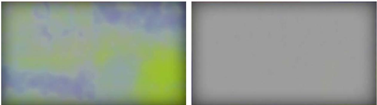
Figure 5: Color of a 46" HDR display for a medium grey input image before (left) and after (right) the correction algorithm is applied. For print reproduction of this paper both image have been adjusted with a 4x saturation enhancement filter. The maximum color variation before adjustment is 14% in the green channel (bottom right corner) and 7% in the blue channel (distributed in several areas across the screen). After calibration all channel are uniform to within less than 1%.
