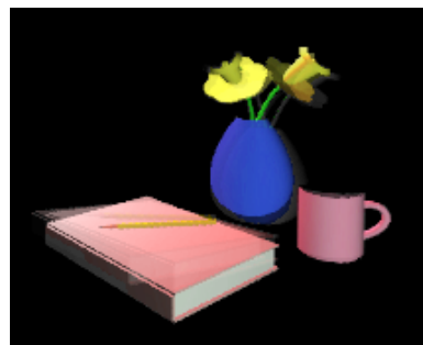
Figure 12: Depth-corrected rendering of the same scene as in Fig. 11, according to the original Lumigraph hardware rendering algorithm [5]. Since the depth rays do not detect all edges, there is still a large amount of blurring.
