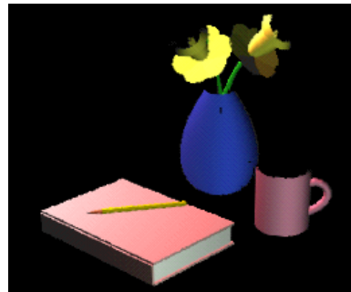
Figure 11: Lumigraph view of a simple scene, computed by warping from 6x6 images of 512x512 pixels resolution.
